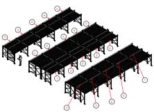
Storage capacity with KLR-12 profiles 25 sections with space for 4500 stereos
