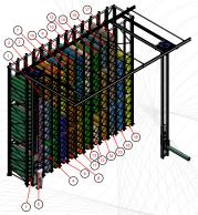
A new developed storage system for 194 pcs Anilox rollers and Printing sleeves.
